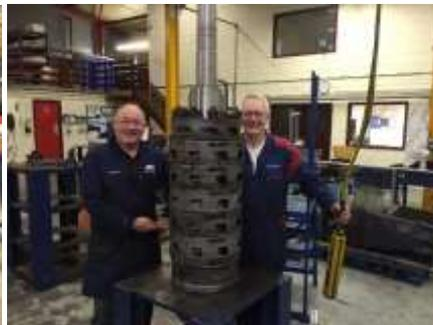
New shaft, stack with seals and complete cartridge assembly with new rotor
