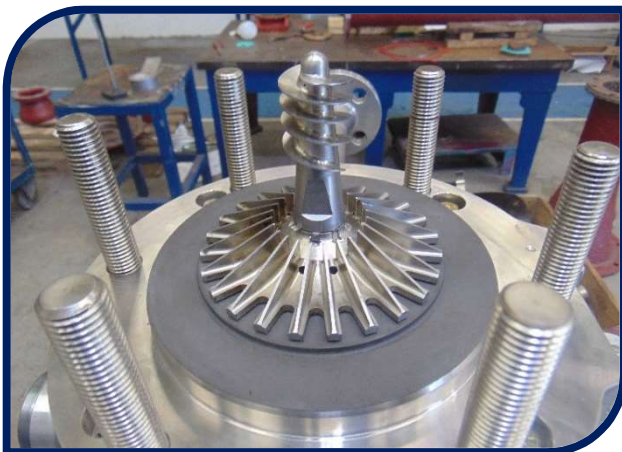
New Impeller machined in-house from Duplex on CNC Machine
