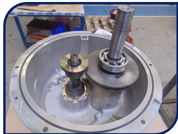
New gears designed and manufactured to re-rate the pump speed
