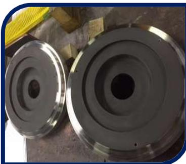
Casing covers and diffuser manufactured in Super Duplex & finished with HVOF Tungsten Carbide
