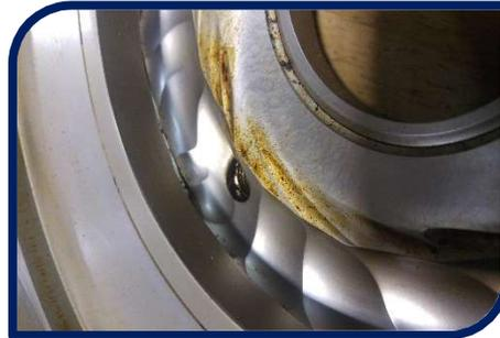
Wash on casing cover through to Mechanical Seal stud holes, creating a leak path and an early failure
