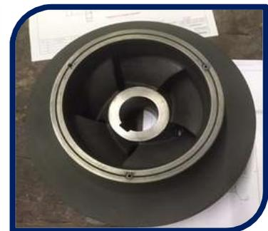
Impeller "line of sight" coated all over in HVOF Tungsten Carbide
