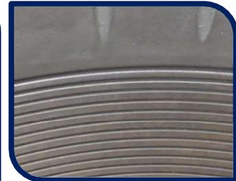
HVOF Tungsten Carbide coating to pressure break down grooves
