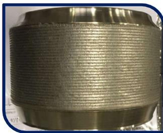
Inter-stage Sleeve, Laser Clad
